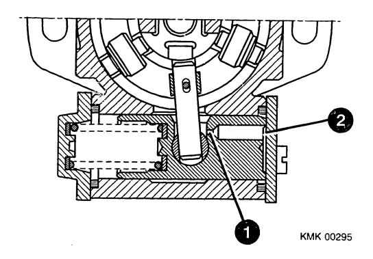
This causes the piston to move to the left against the spring force. A higher internal pump pressure results in "advance" and a lower pressure in "retard". **80H** - 5 -
